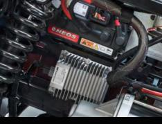
Toyota Industries-built motor controller unit.
